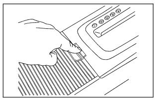
There are two removable cupholders and additional storage areas located at the rear of the shift lever. To access, push the button and the cover will slide back automatically. To close, slide the cover forward and lock into place.
